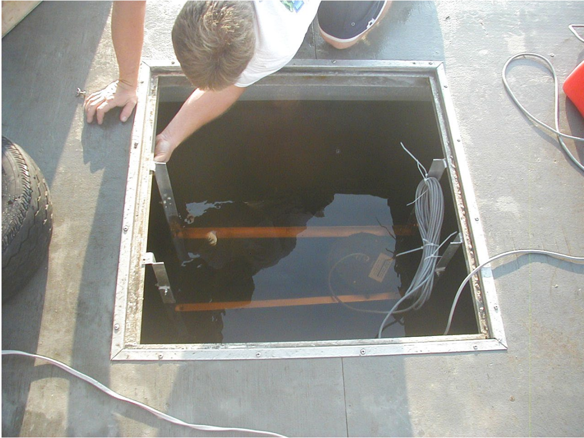
Figure 6. The survey echo sounder was mounted at 18 cm below water surface.
