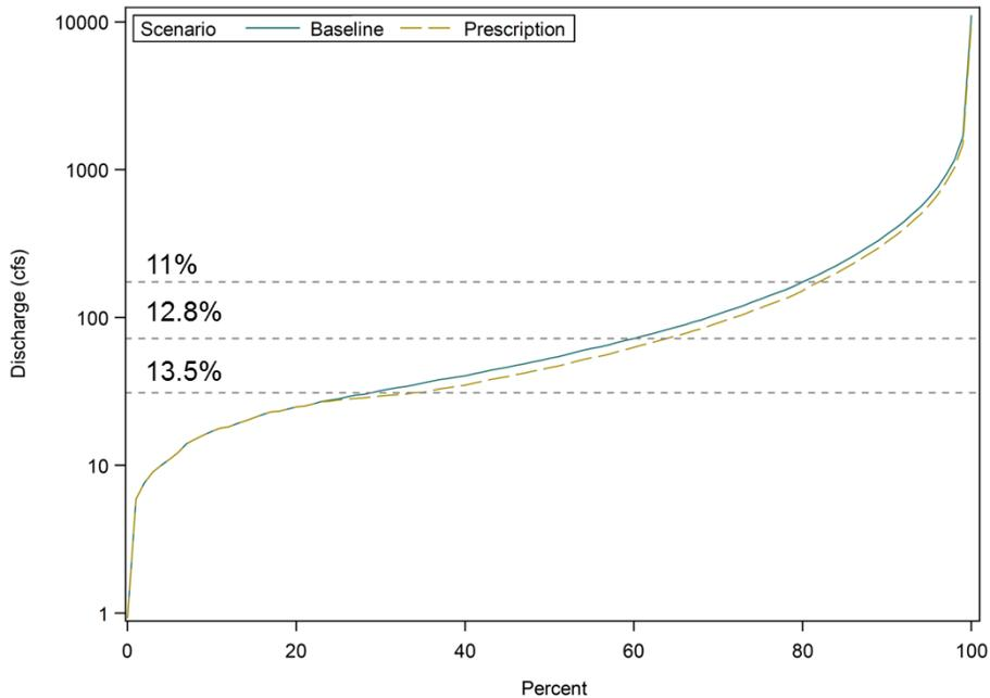
**Figure 7-1. Baseline and Prescription flow distribution with allowable consumptive use located on the hydrograph.**
