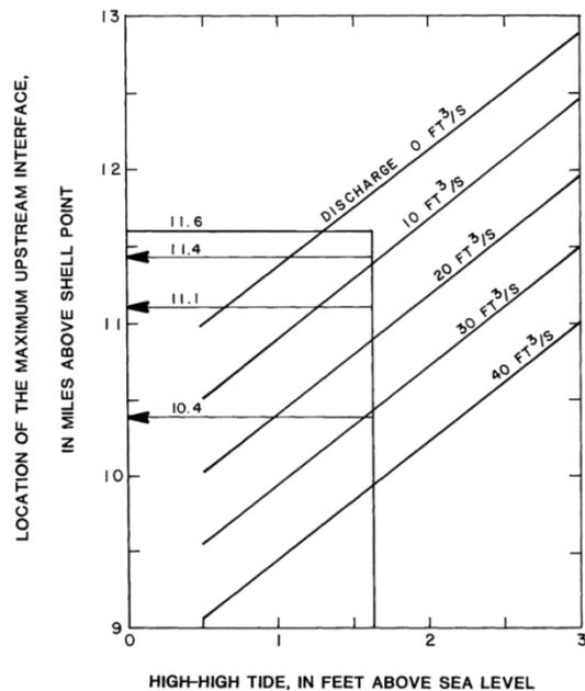
**Figure 3-21. Estimated location of the freshwater interface as a function of tide and discharge from USGS02300500-Wimauma as reported in Figure 22 of Fernandez 1985. Note that location is described in river miles in this figure.**
