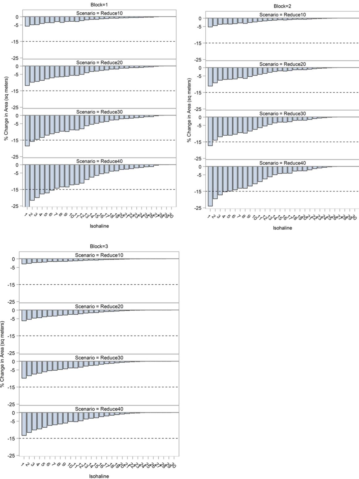
**Figure 5-5. Percent change (y axis) in bottom area (square meters) for salinity isohalines less than 1 through 30 (x axis) BY BLOCK. Broken reference line represents 15% threshold used to identify potential for significant harm.**
