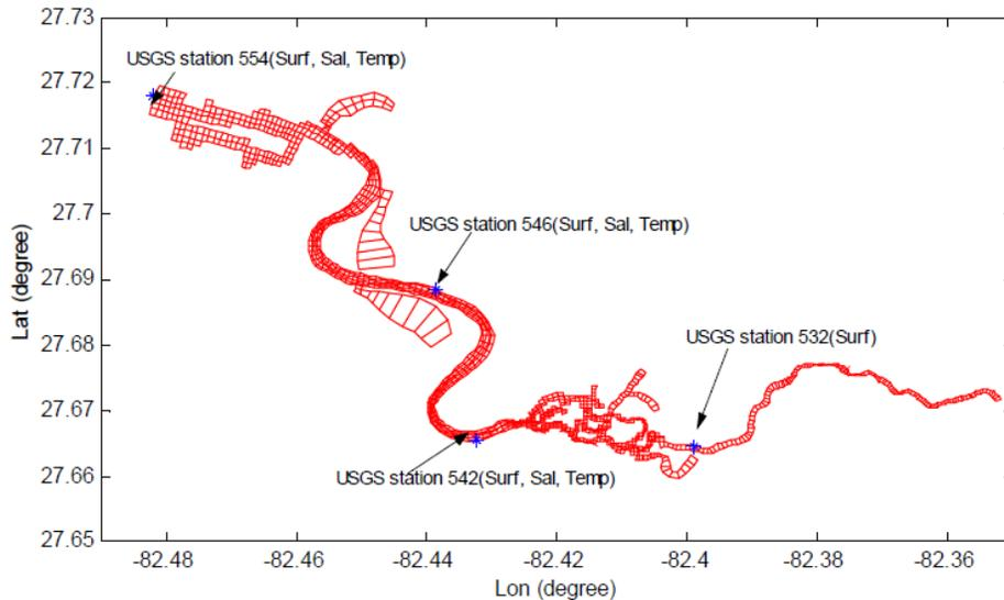
**Figure 3-11. Model grid used by the EFDC model for the tidal reach of the Little Manatee River.**
