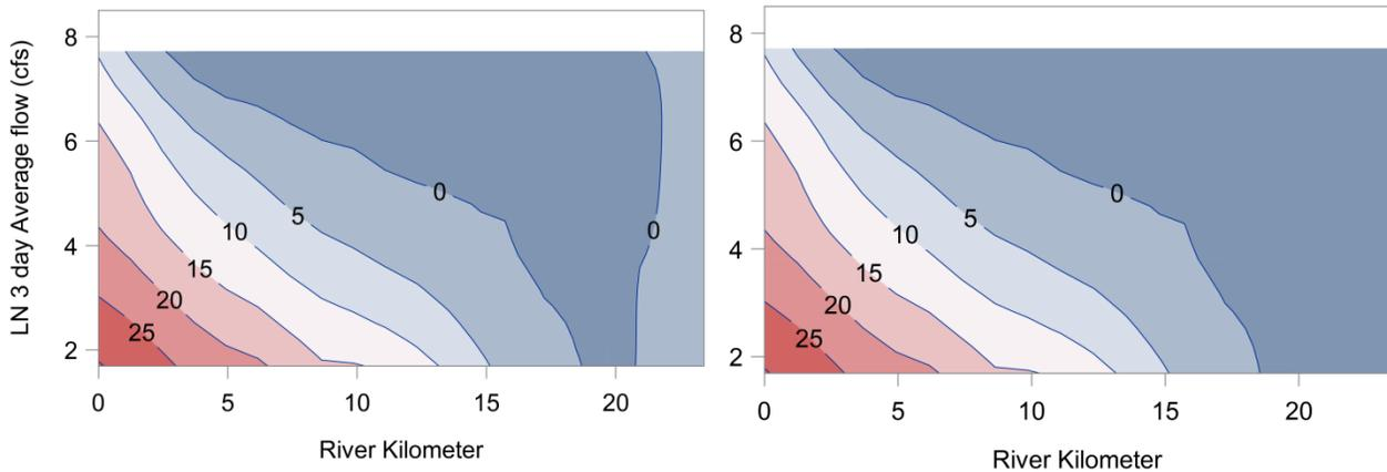
**Figure 3-20. Contour plot of water column average salinity based on empirical data update with (left) and without (right) the three observations in Table 3-5.**
