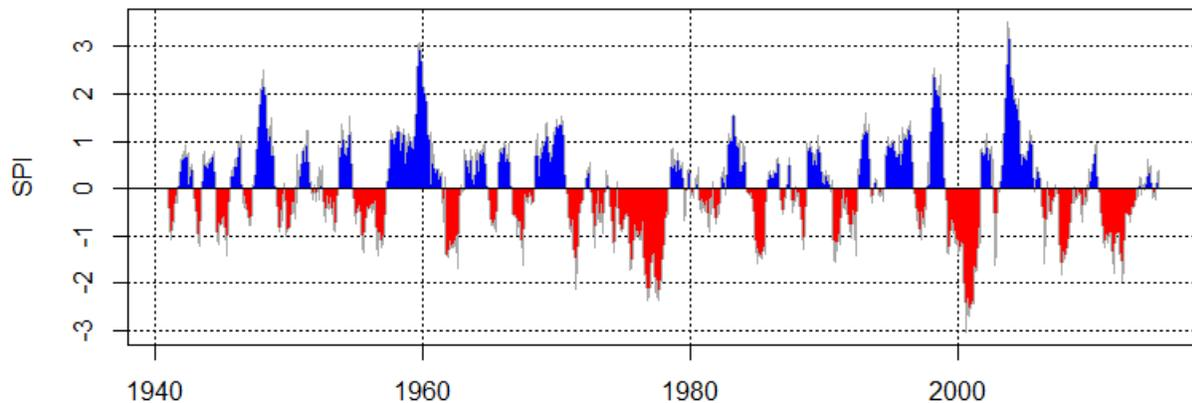
**Figure 2-3. Twelve month Standardized Precipitation Index values for the Parrish gage based on data from 1940 to 2014.**
