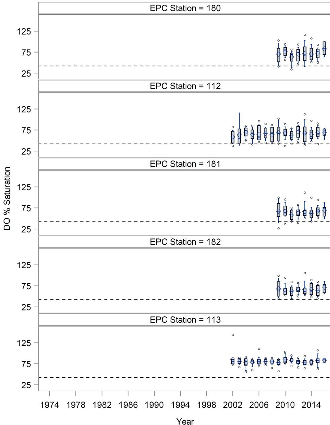
Figure 3-28. Annual distribution of dissolved oxygen expressed as percent saturation. Broken horizontal reference line represents FDEP threshold criteria for evaluating impairment based on narrative standard.
