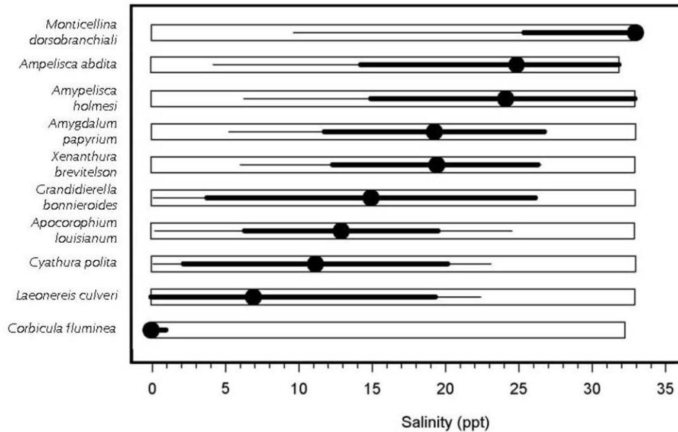
**Figure 4-3.** Summary of salinity optimum (circle), optimal habitat range (i.e., 75% of optimum solid bar), 10<sup>th</sup> to 90<sup>th</sup> percentile probability of occurrence (thin line), and salinity model domain (open bar) for ten selected benthic taxa using pooled data from 12 southwest Florida tidal rivers (wet and dry seasons combined).
