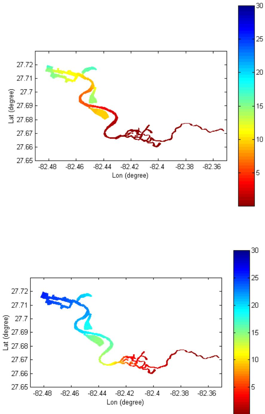
**Figure 3-12. Salinity field at low tide (top) and high tide (bottom) on 2/9/2005 under river flow of 52 cfs.**
