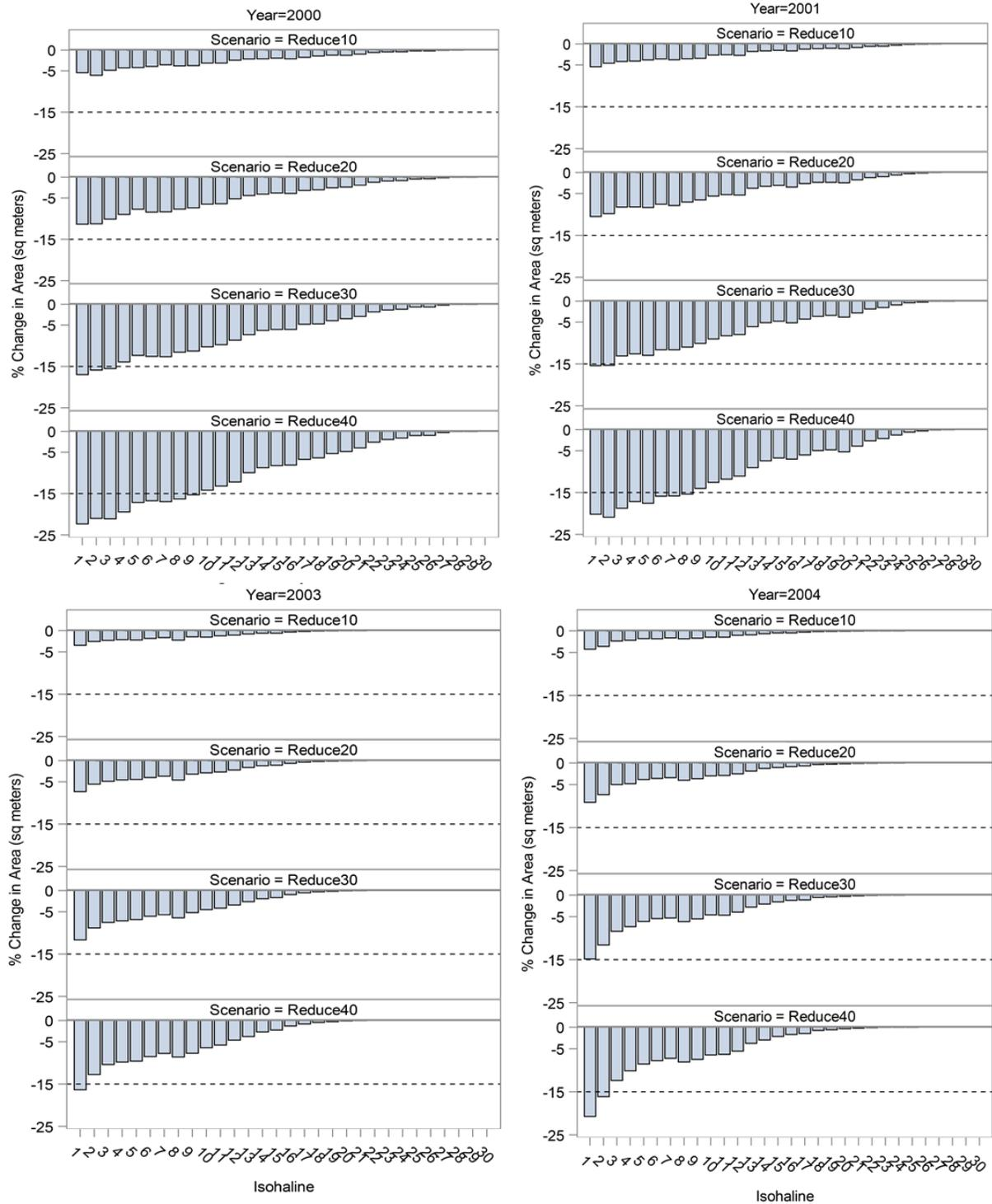
**Figure 5-4. Percent change (y axis) in bottom area (square meters) of salinity isohalines less than 1 through (less than) 30 (x axis) BY YEAR. Broken reference line represents 15% threshold used to identify potential for significant harm.**
