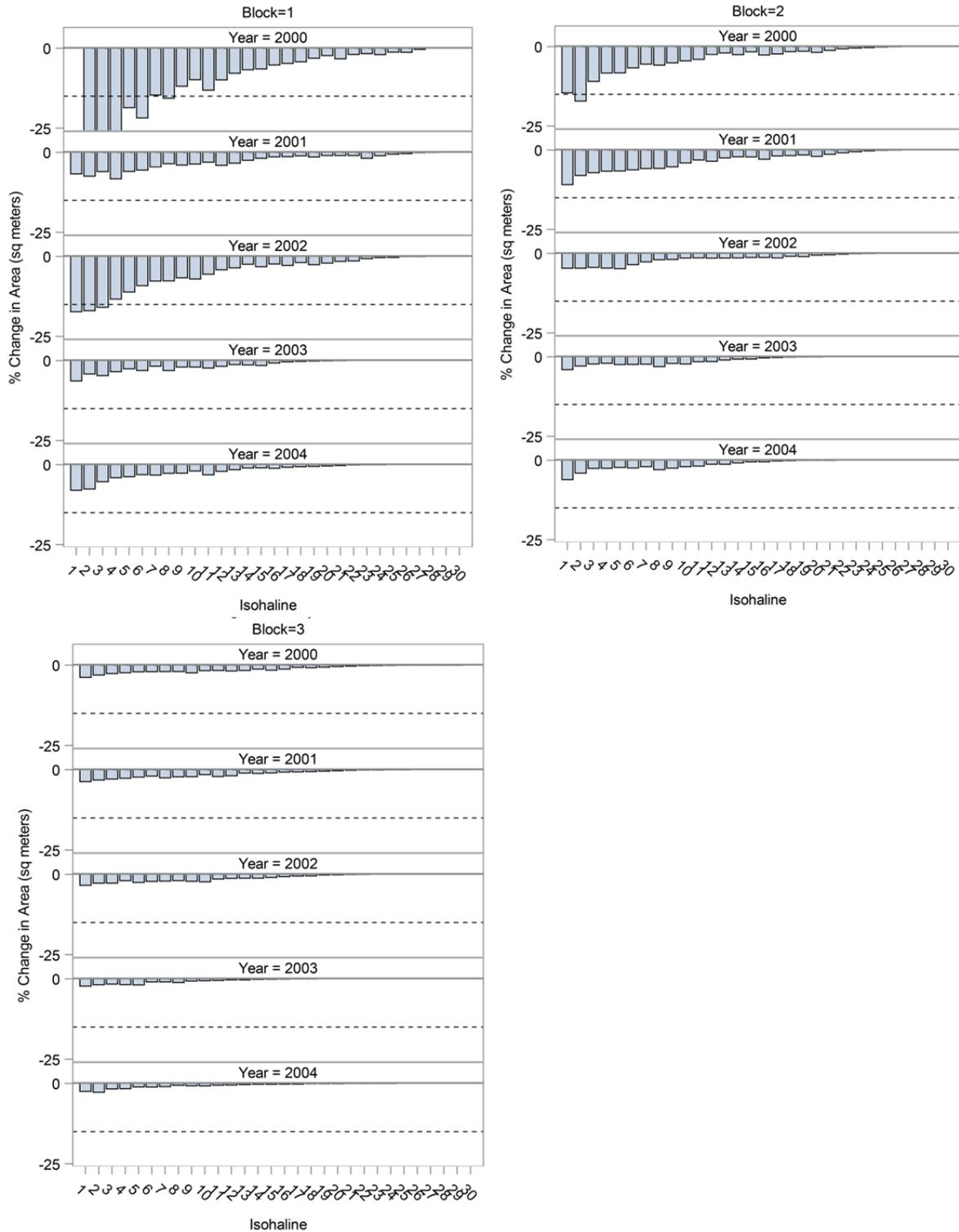
**Figure 5-6. Percent change (y axis) in bottom area (square meters) for salinity isohalines less than 1 through 30 (x axis) BY YEAR AND BLOCK for the 10% reduction scenario only. Broken reference line represents 15% threshold used to identify potential for significant harm.**
