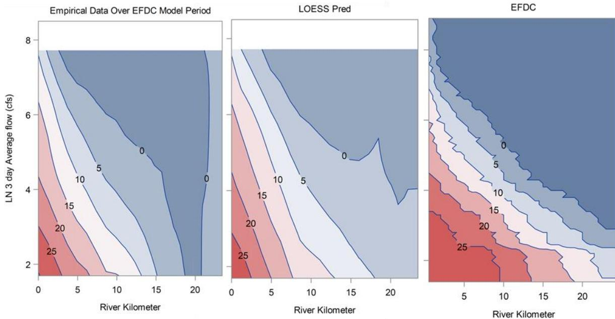
**Figure 3-24. Contour plots of empirical data (left), LOESS regression predictions (middle), and EFDC model predictions (right) over the EFDC model time domain. Note that no flow values higher than 7.8 (log scale) were observed in combination with empirical synoptic data collections over the EFDC model period and therefore the white space at the top of the two graphs on the left.**
