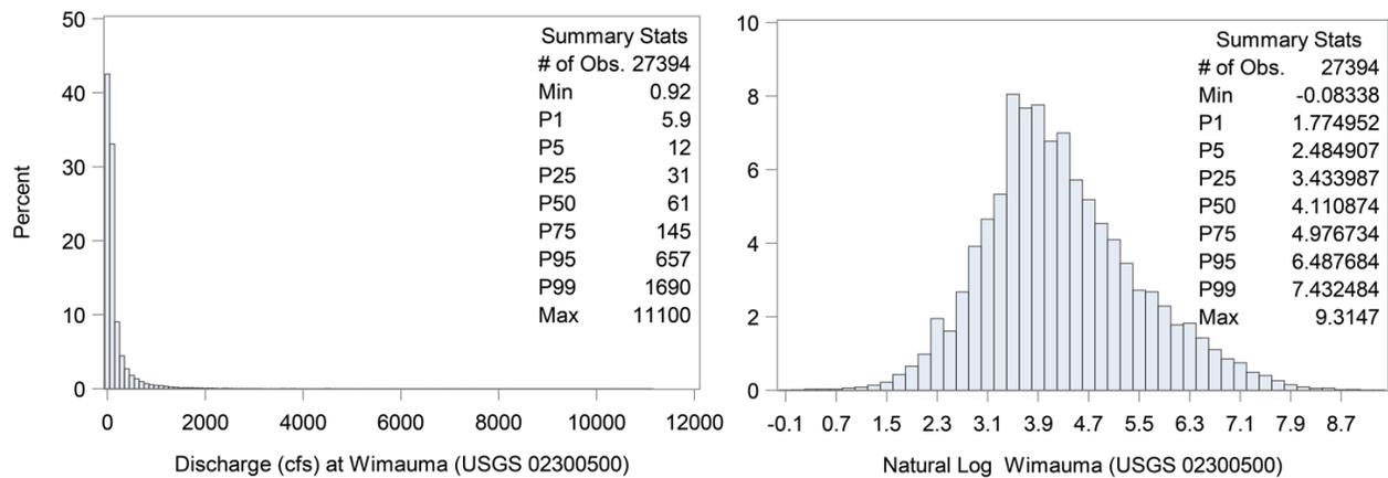
**Figure 2-5. Frequency histogram and summary statistics for discharge at USGS 02300500 – Wimauma from 1940 through 2014 on natural (left) and natural log transformed (right) scale.**
