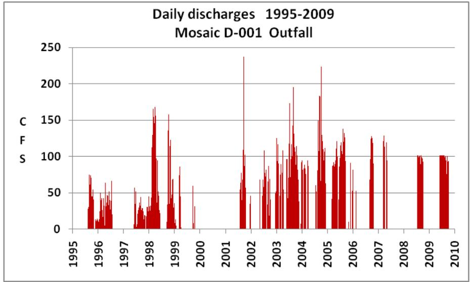
Figure 2-7. Figure 4-16 from Hood et. al., 2011 displaying daily discharge values for the D-001 outfall through 2009.
