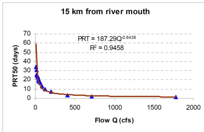
**Figure 3-14. Pulse Residence Times as a function of flow for the 17 flow values evaluated.**
