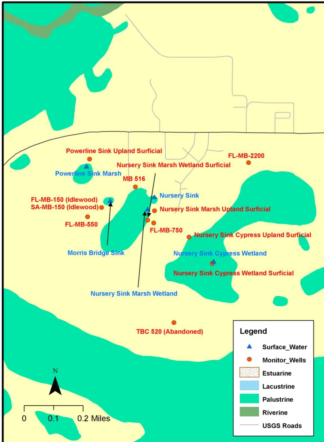
Figure 4. Location of Monitor Wells and Surface Water Stage Recorders used in the Morris Bridge Sink Pumping Test.
