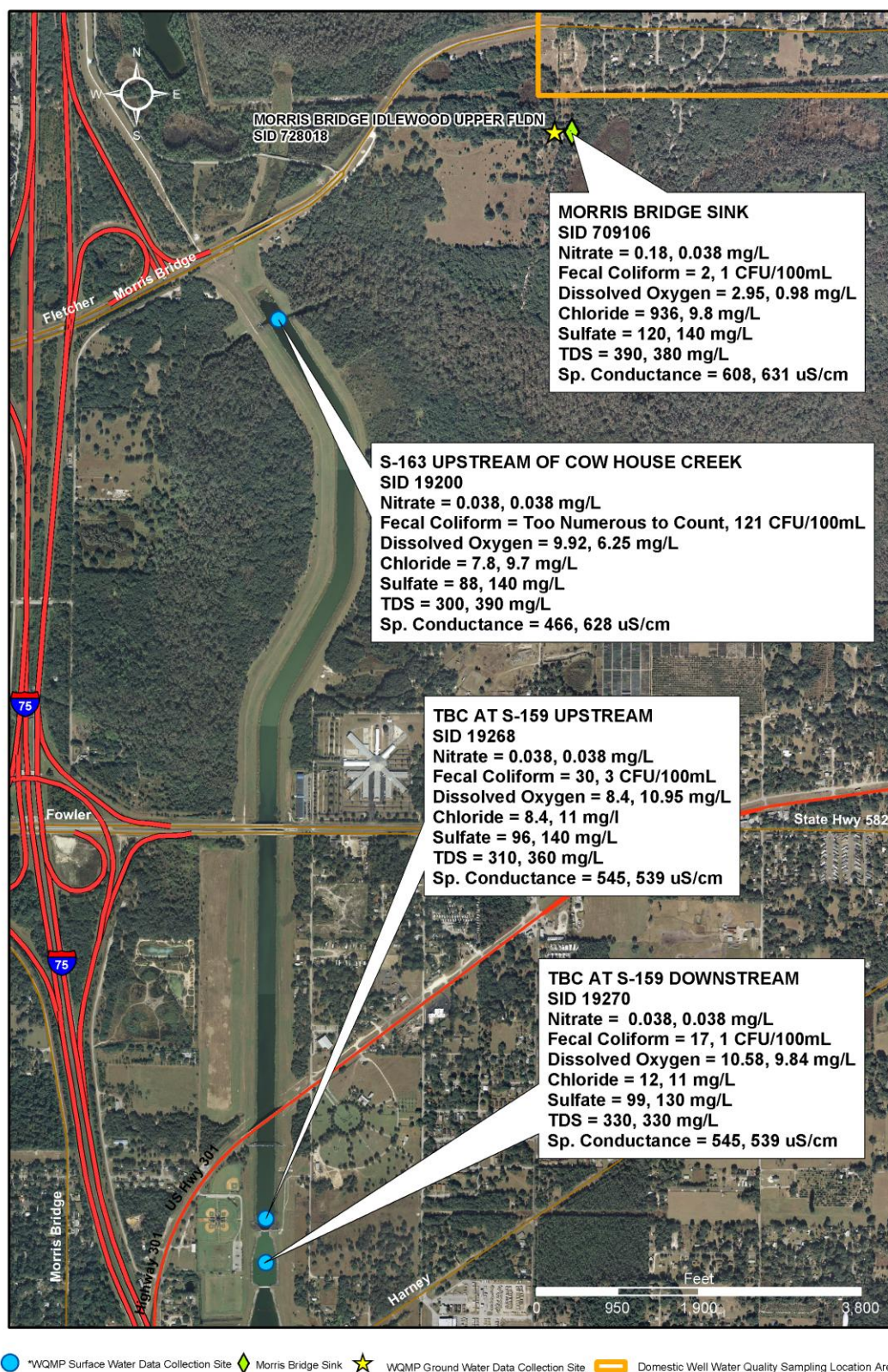
Figure 32. Select water quality parameters collected from Morris Bridge Sink pumping test during the baseline and final sampling events.
