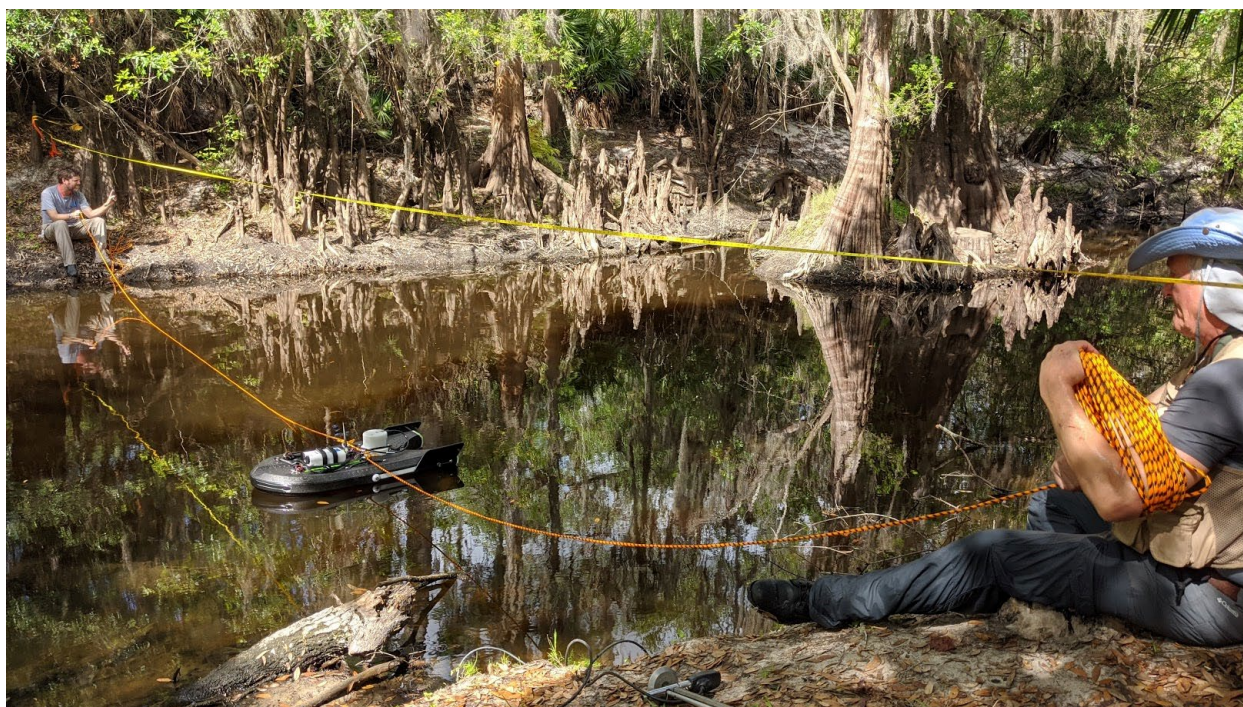
Figure 3. Moving boat discharge measurements on Charlie Creek.
