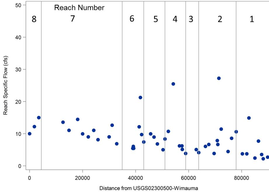
**Figure 4-4. Reach specific critical flow values associated with a 0.6-foot hydrologic depth for fish passage in the Upper Little Manatee River. See Figure 3-9 for river reach delineations.**
