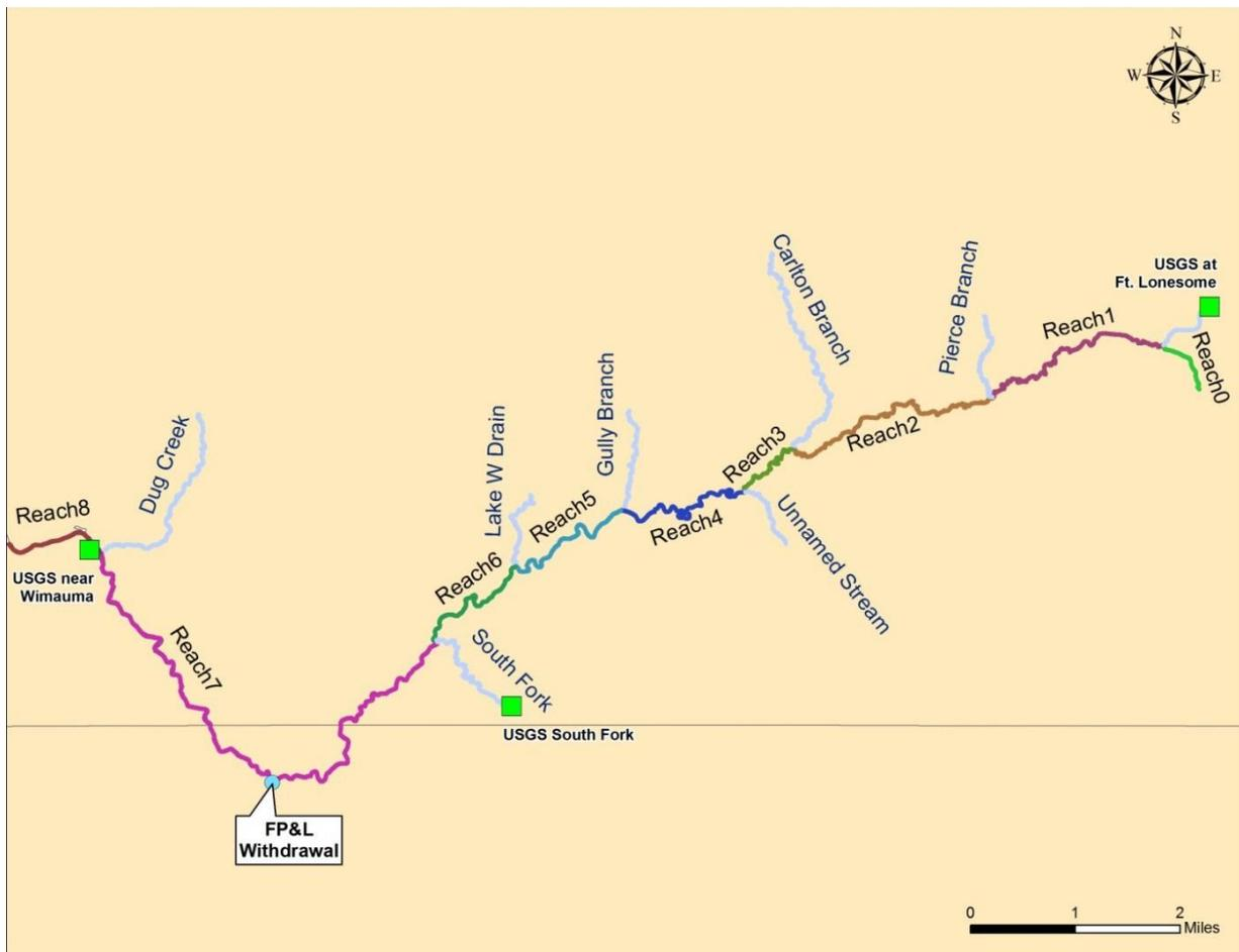
**Figure 3-6. HEC-RAS model reaches, USGS gages and principal utility with a surface water withdrawal permit in the Upper Little Manatee River.**
