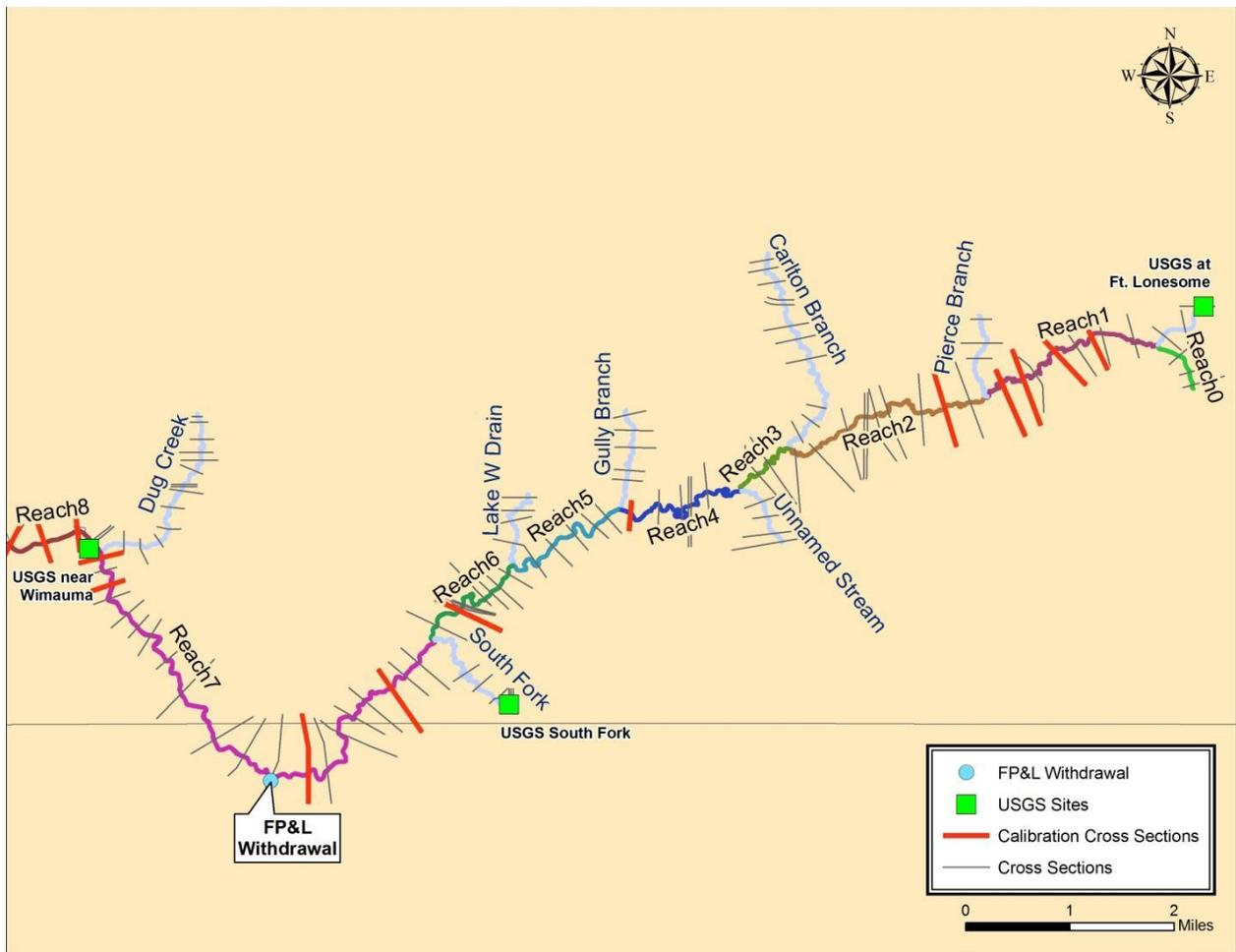
**Figure 3-8. SWMM model cross sections imported into HEC-RAS for model update for the Upper Little Manatee River. The red lines indicate the 15 SWMM calibration cross sections used to recalibrate the HEC-RAS model.**
