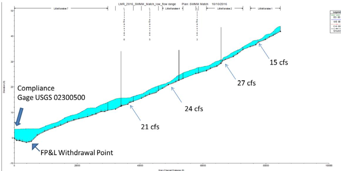
**Figure 4-5. Water-surface profile of the main stem of the Little Manatee River with critical shoals for fish passage denoted by arrows and labeled with reach specific flow requirements necessary to maintain hydrologic depth of 0.6 feet.**
