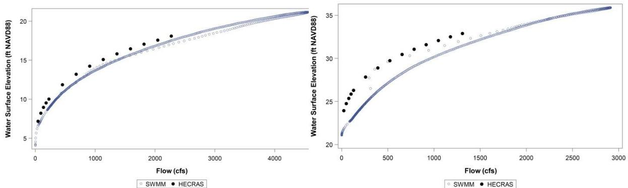
**Figure 2-10. Comparison of flow stage curves at two locations in the Little Manatee River above US 301, near the USGS gage (left) and far upstream of the gage (right). The HEC-RAS model prediction is represented by the black filled circle and SWMM model prediction represented by the blue open circles.**
