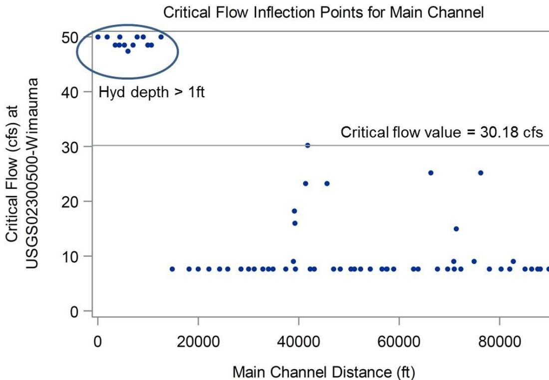
Figure 4-2. Critical flow for each HEC-RAS cross section (y axis) as a function of distance from the downstream flow gage (USGS02300500).
