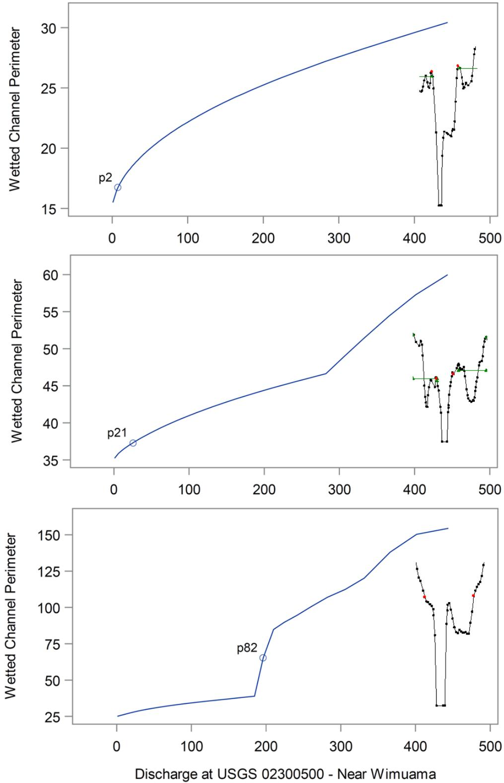
**Figure 4-1. Wetted-perimeter curves as a function of flow at the USGS02300500, Little Manatee River near Wimauma, FL gage. Insets are entire cross section (lower right) and expanded view of channel center geometry (upper left).**
