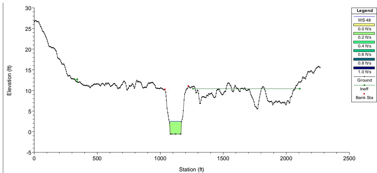
**Figure 4-3. Example cross-section (115.66) in the upper Little Manatee River where the inflection point was associated with a relatively deep channel water depth (i.e., 3.07 feet).**
