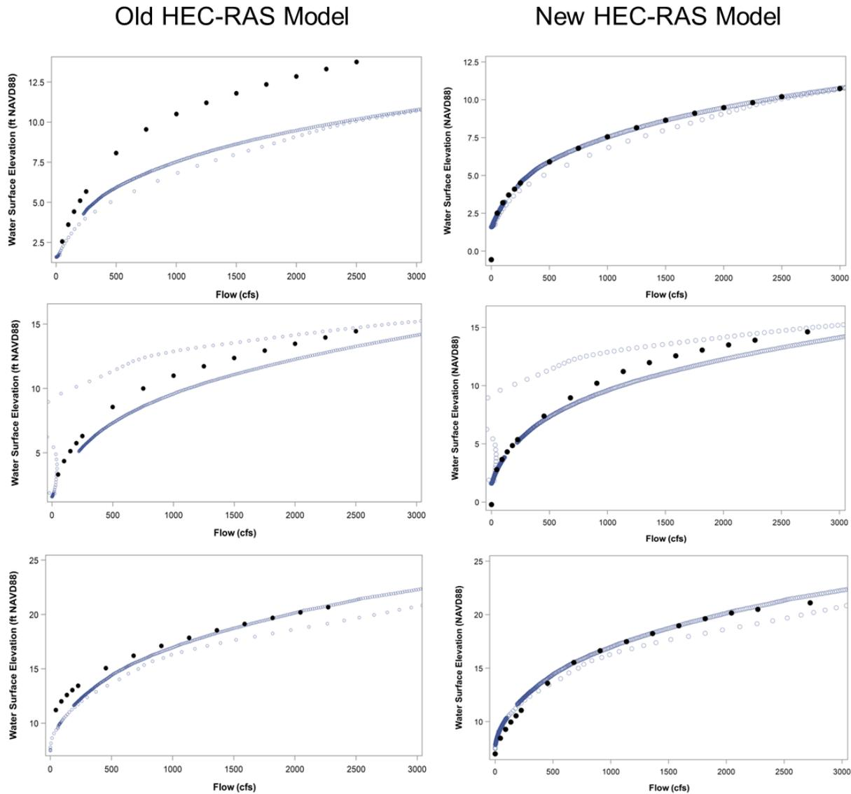
**Figure 3-9. HEC-RAS and SWMM model comparisons for the original Upper Little Manatee HEC-RAS model (left) and recalibrated HEC-RAS model (right) at three representative cross sections.**
