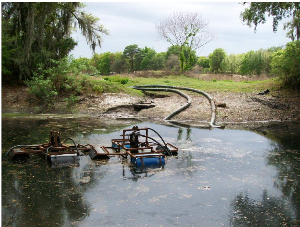
Figure 4. Pumps and discharge lines used in the Blue Sink test.
