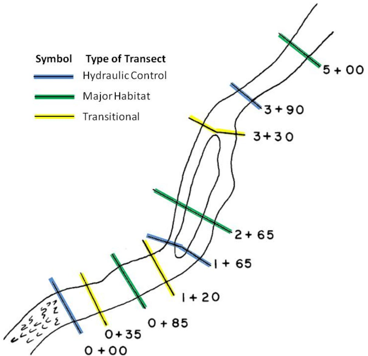
Figure 6. Example PHABSIM transects and configurations for characterization of stream study sites (adapted from Bovee and Milhous 1978).
