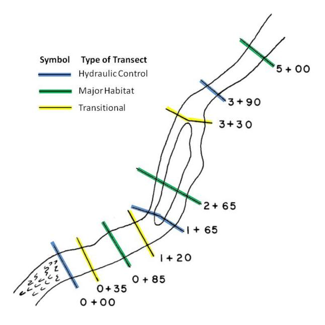
Figure 6. Example PHABSIM transects and configurations for characterization of stream study sites (adapted from Bovee and Milhous 1978).
