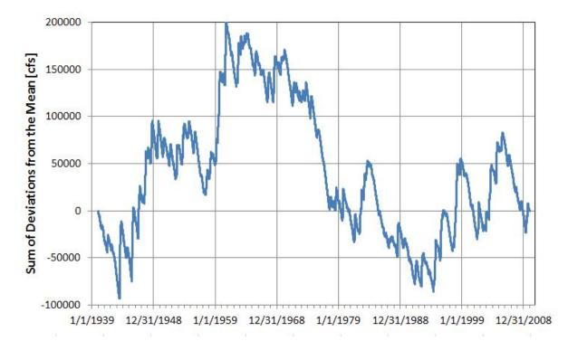
Figure 7. Cumulative departures from the mean for average daily flow at the Little Manatee River near Wimauma, FL (USGS gage 02300500).
