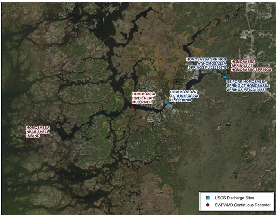
**Figure 2-5. Water quality continuous recorders (red circles) on the Homosassa River. Blue squares indicate the locations of USGS river discharge gages.**
