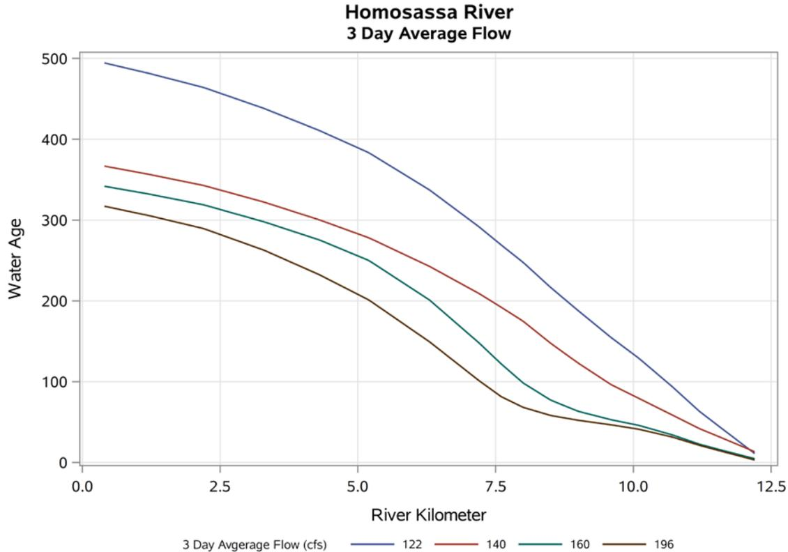
**Figure 3-19. Water age (in hours) curves for four different 3 day average flows.**
