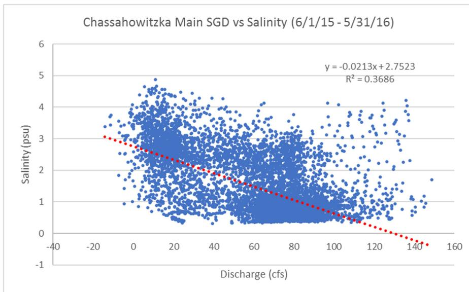
Figure 9. SGD versus salinity at the USGS Chassahowitzka River near Homosassa station during the 12-month period of June 1, 2015 through May 31, 2016.
