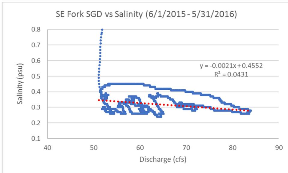
Figure 12. Plot of tidally filtered SGD versus tidally filtered salinity at the USGS SE Fork station during the 12-month period of June 1, 2015 through May 31, 2016.
