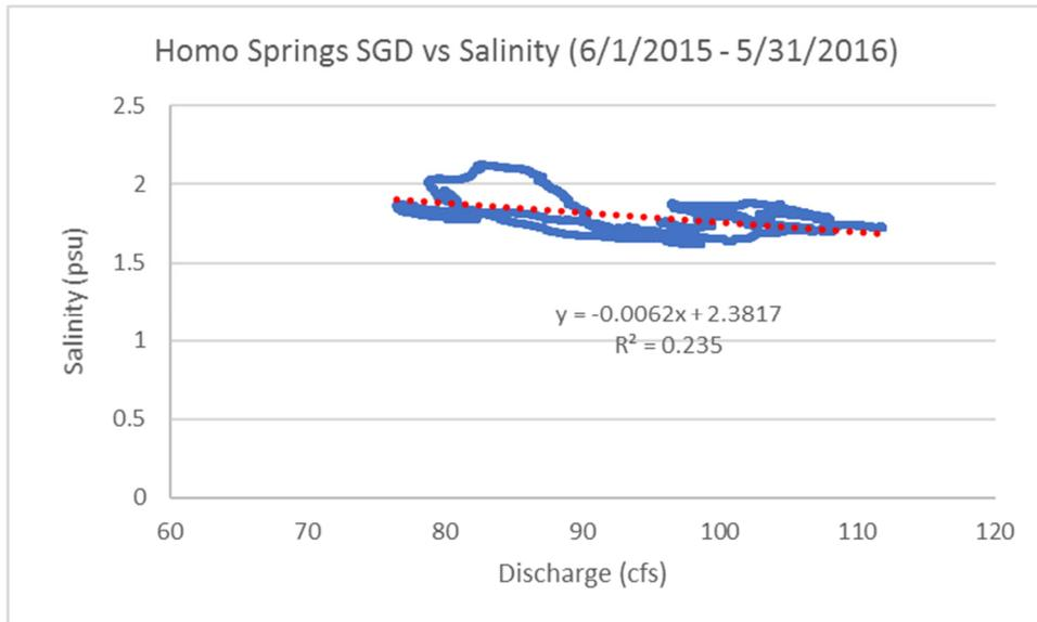
Figure 13. Plot of tidally filtered SGD versus tidally filtered salinity at the USGS Homosassa Springs station during the 12-month period of June 1, 2015 through May 31, 2016.
