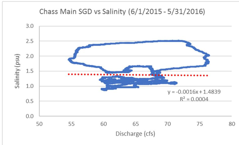
Figure 15. Tidally filtered SGD versus tidally filtered salinity at the USGS Chassahowitzka River near Homosassa station during the 12-month period of June 1, 2015 through May 31, 2016.
