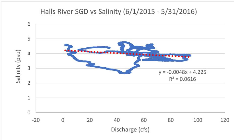
Figure 14. Plot of tidally filtered SGD versus tidally filtered salinity at the USGS Halls River at Homosassa Springs station during the 12-month period of June 1, 2015 through May 31, 2016.
