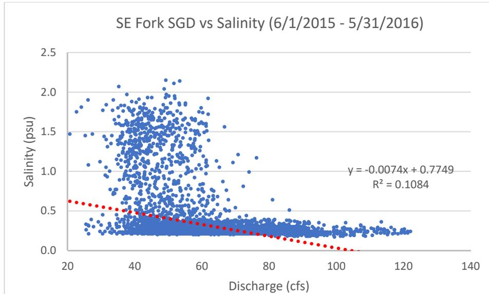
Figure 5. Plot of SGD versus salinity at the USGS SE Fork station during the 12-month period of June 1, 2015 through May 31, 2016.
