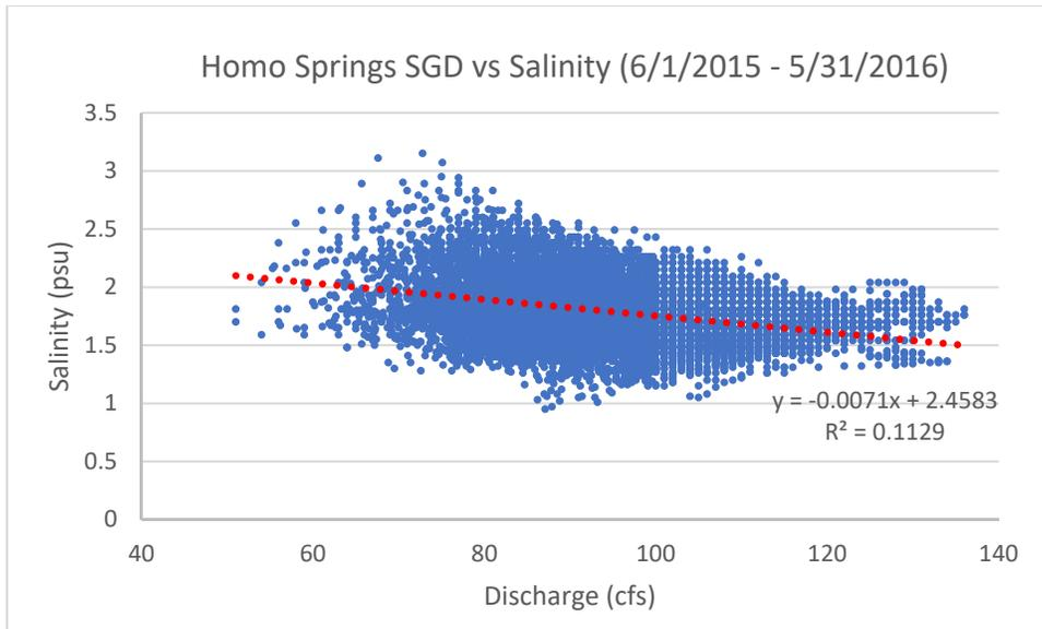
Figure 6. Plot of SGD versus salinity at the USGS Homosassa Springs station during the 12-month period of June 1, 2015 through May 31, 2016.
