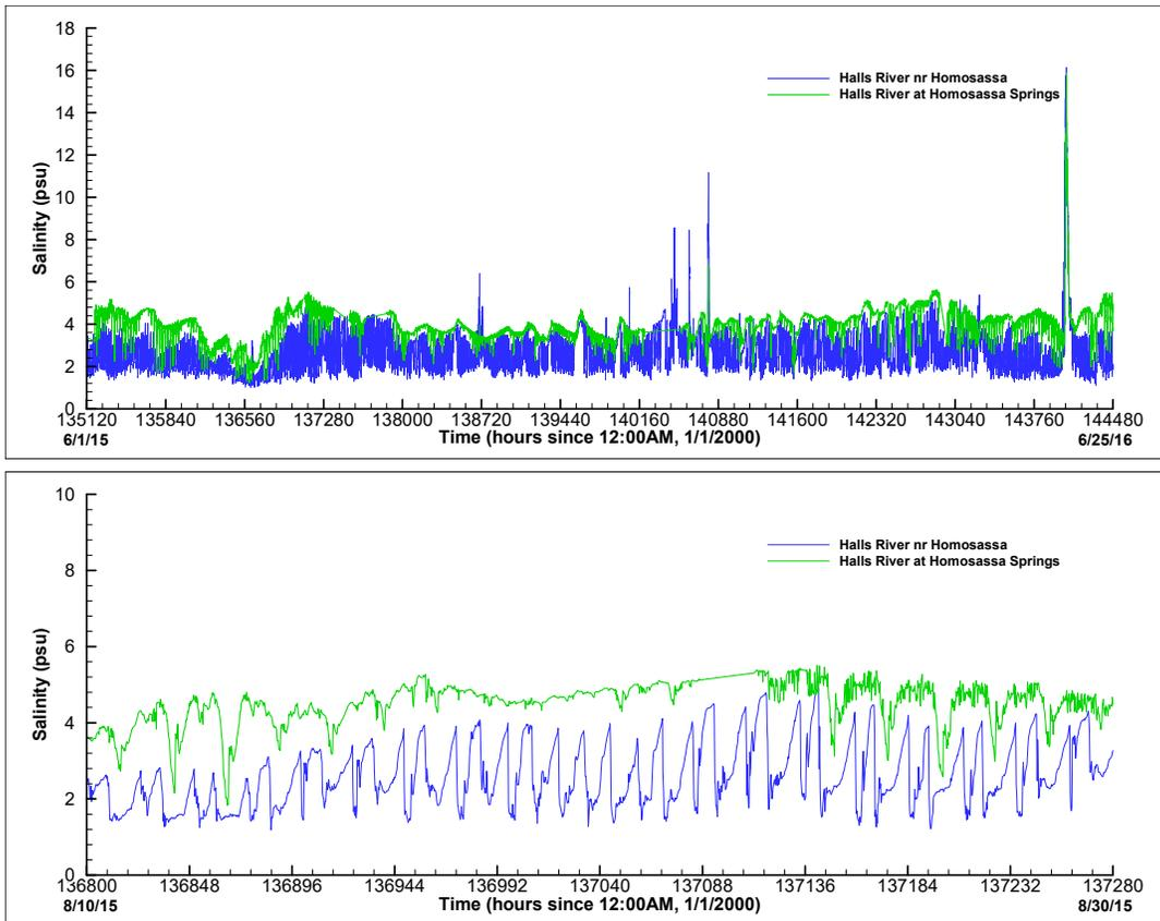
Figure 8. Measured salinities at the Halls River near Homosassa (blue lines) and Halls River at Homosassa Springs (green lines) stations during June 1, 2015 through June 25/2016.
