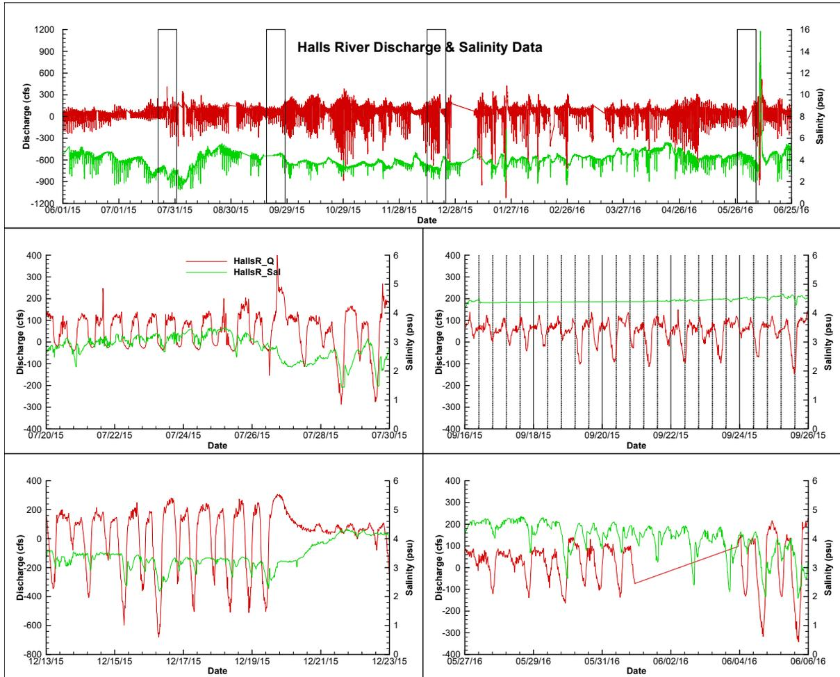
Figure 3. Discharge (red lines) and salinity (green lines) data collected at the USGS Halls River at Homosassa Springs station during June 1, 2015 through June 25, 2016 (top panel). Data for four 10-day windows (7/20/15 – 7/30/15, 9/16/15 – 9/26/15, 12/13/15 – 1/23/16, and 5/27/16 – 6/6/16) were plotted in the middle and bottom four panels.
