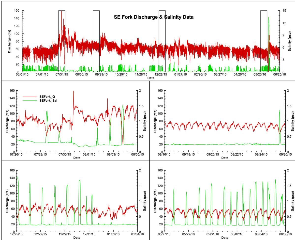
Figure 1. Discharge (red lines) and salinity (green lines) data collected at the USGS SE Fork station during June 1, 2015 through June 25, 2016 (top panel). Data for four 10-day windows (7/20/15 – 7/30/15, 9/16/15 – 9/26/15, 12/23/15 – 1/2/16, and 5/31/16 – 6/10/16) were plotted in the middle and bottom four panels.
