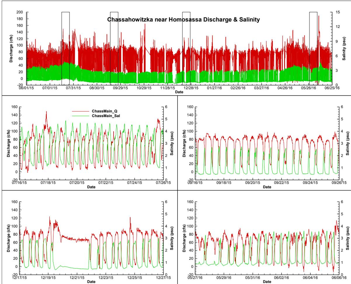
Figure 4. Figure. Discharge (red lines) and salinity (green lines) data collected at the USGS Chassahowitzka River near Homosassa station during June 1, 2015 through June 25, 2016 (top panel). Data for four 10-day windows (7/16/15 – 7/26/15, 9/16/15 – 9/26/15, 12/17/15 – 12/27/15, and 5/27/16 – 6/06/16) were plotted in the middle and bottom four panels.
