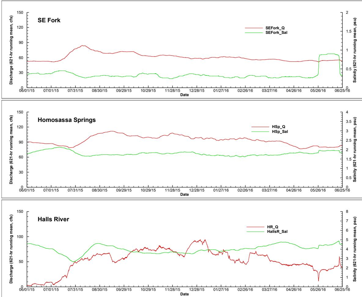
Figure 10. 621-hour running means of discharge (red lines) and salinity (green lines) at the USGS SE Fork (top panel), Homosassa Springs (middle panel), and Halls River at Homosassa Springs (bottom panel) stations during June 1, 2015 through June 25, 2016.
