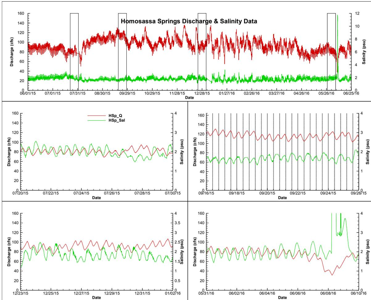
Figure 2. Discharge (red lines) and salinity (green lines) data collected at the USGS Homosassa Springs station during June 1, 2015 through June 25, 2016 (top panel). Data for four 10-day windows (7/20/15 – 7/30/15, 9/16/15 – 9/26/15, 12/23/15 – 1/2/16, and 5/31/16 – 6/10/16) were plotted in the middle and bottom four panels.
