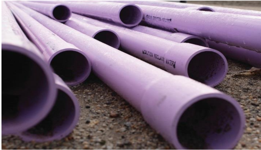
Reclaimed water pipes
