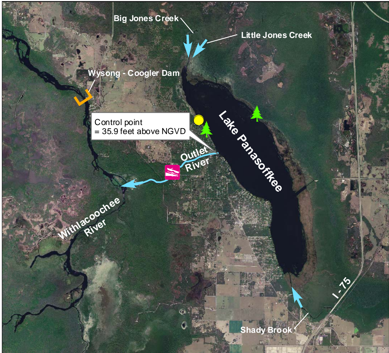
Figure 2. Location of the lake water level gauge, public boat ramps, hydrologic indicators, inlets, outlet, outlet conveyance system, water control structure, and control point for Lake Panasoffkee.
