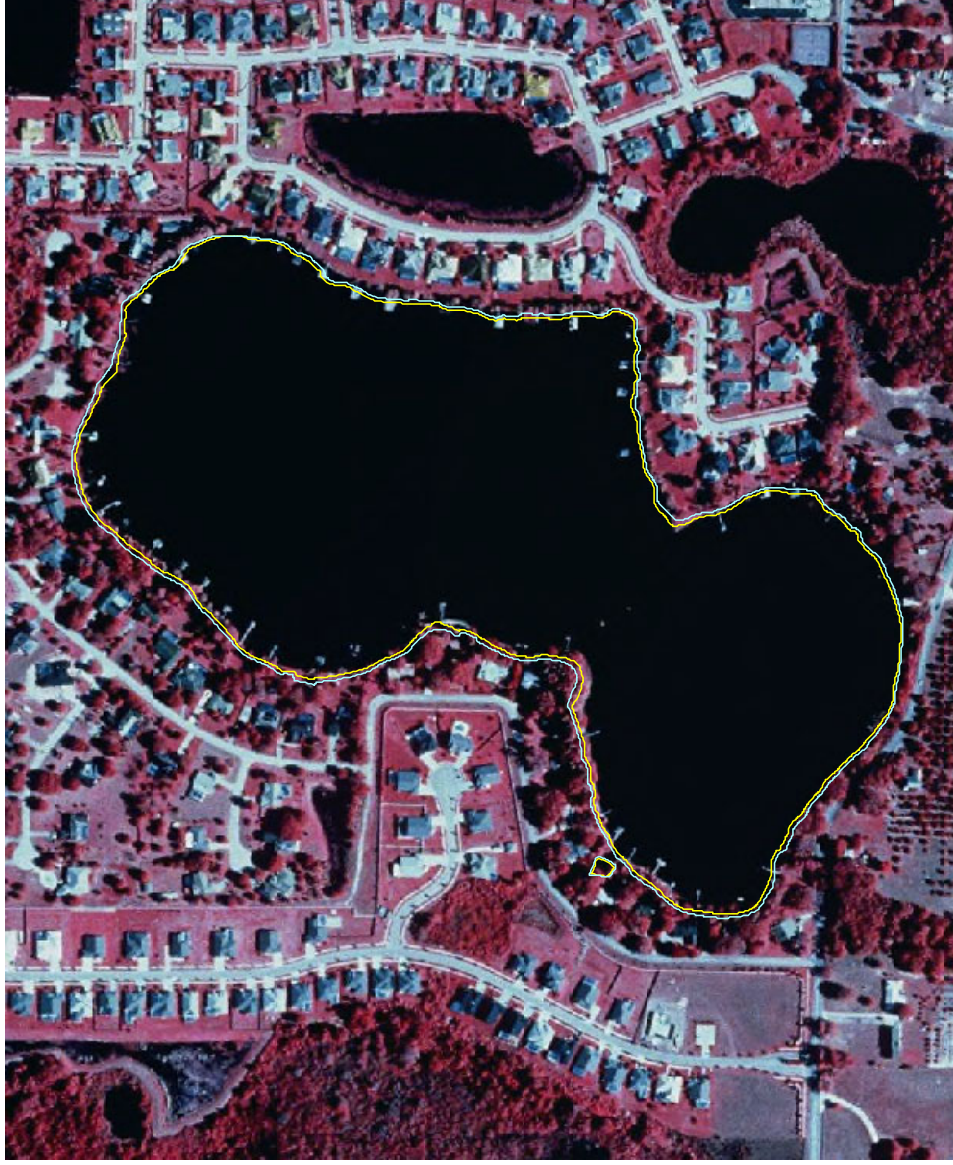
Figure Fairy-4. Approximate location of the proposed Minimum Lake Level (yellow) and the proposed High Minimum Lake Level (blue) for Fairy Lake, Hillsborough County, Florida. Elevations listed are in feet, relative to the National Geodetic Vertical Datum of 1929.
