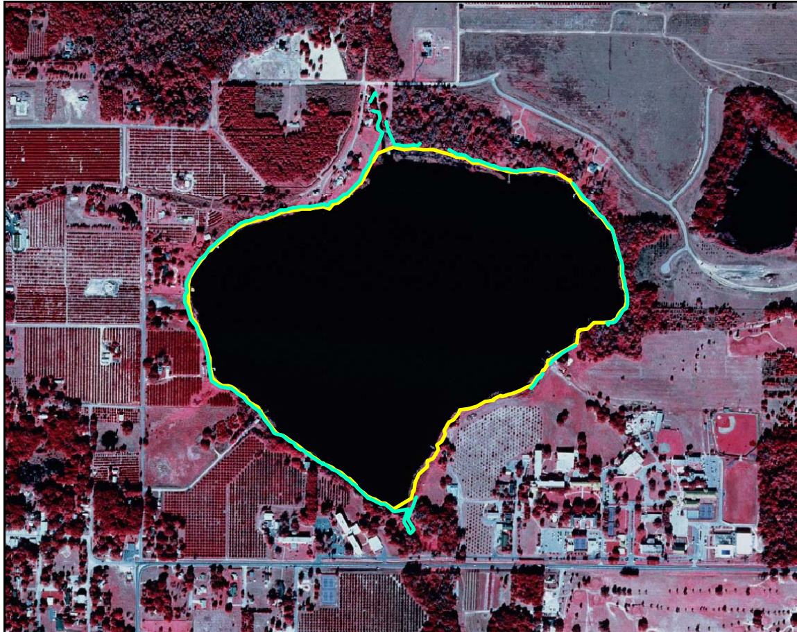
Figure 4. Approximate location of the proposed Minimum Lake Level (yellow) and proposed High Minimum Lake Level (blue) for Clear Lake in Pasco County, Florida. Elevations of contours are in feet above the National Geodetic Vertical Datum of 1929.
