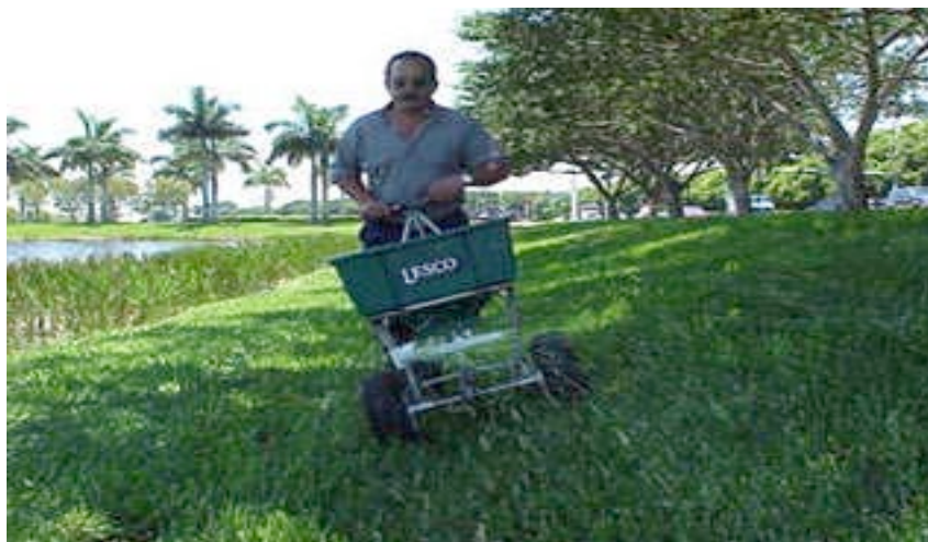
A fertilizer spreader that features a deflector shield to deflect fertilizer granules away from all impervious surfaces, fertilizer-free zones and water bodies, including wetlands, is a provision of the model ordinance developed and recommended by the Task Force.
