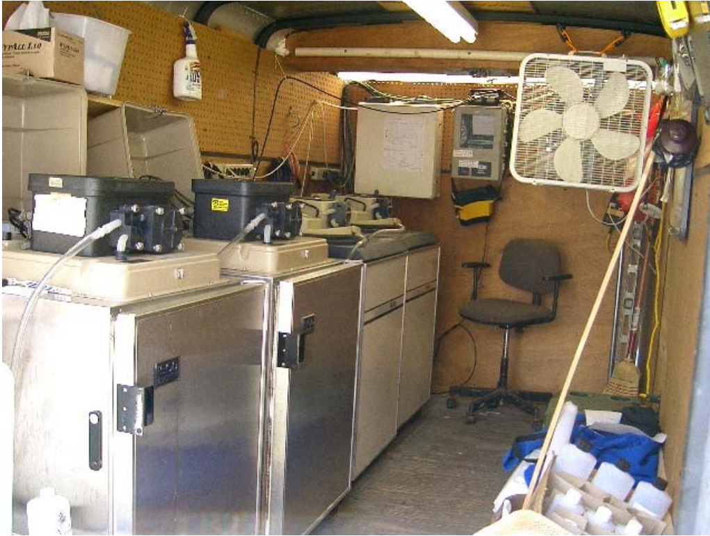
View of instrument trailer showing four refrigerated samplers for collecting storm flow and base flow samples. The CR10 and ISCO water level sensor is shown on the back wall.
