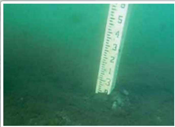
Organic sediment accumulation in the upper Homosassa River is caused by detritus settling out from the water column as flow declines. Organic sediment thickness can be as much as 4-feet thick in the upper reaches of the river.
