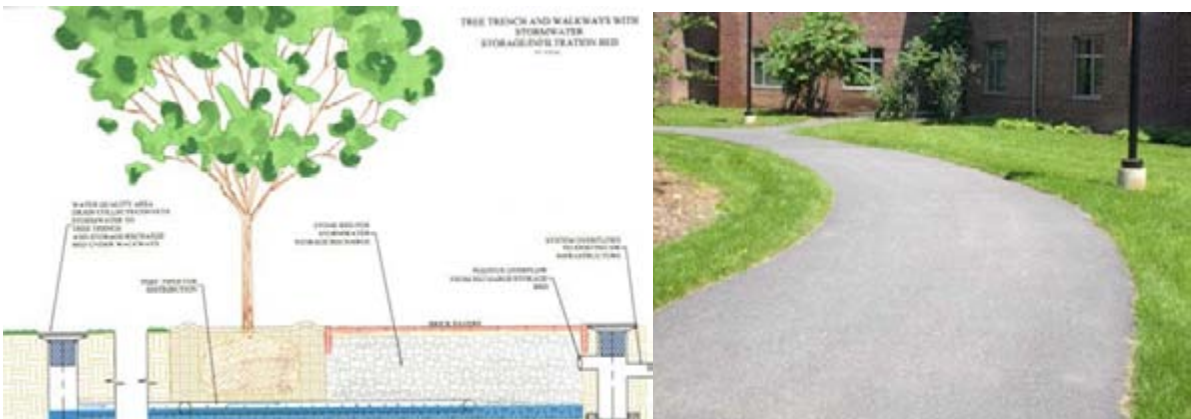
Infiltration Beds beneath Asphalt Paths with Grasspave along Edges for Fire Access
