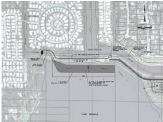
Figure 13. Alum injection and in-lake flocculent settling area for Sub-basin 1.
