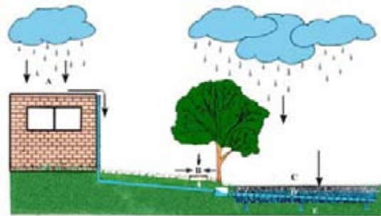
Roof Leaders convey runoff to stormwater bed below playfield.
