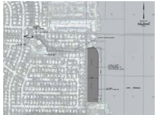
Figure 13 Alum injection and in-lake flocculent settling area for Sub-basin 2.
